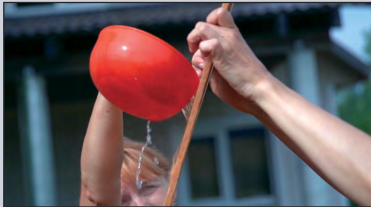
Hot water is poured over the lake soaked boards to help them bend
