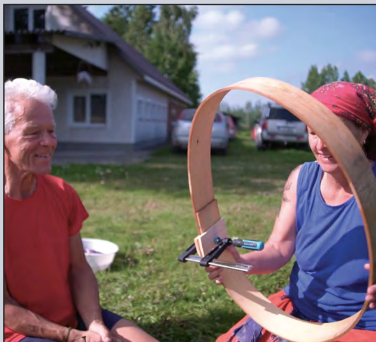
The freshly bent drum hoop is clamped so the two ends can be joined
