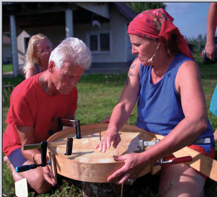
Bending the boards around a former to help give them shape
